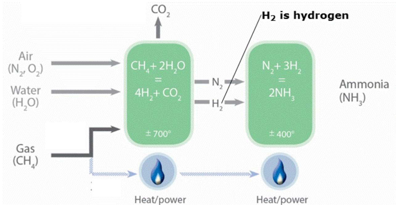
Figure 2: Simplified ammonia production process [adjusted from figure received from Fertilizers Europe]
